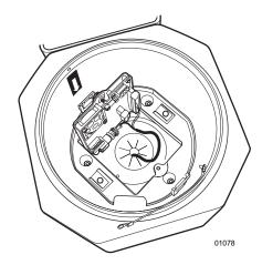
c. Thread the cable/wiring through the back box mounting plate. Attach the plate to the mounting base using the screws previously removed. Pull cable/wiring into the inside back box (the back box hinged door should be opened). Attach the inside back box to the mounting plate. Use the three Phillips head screws previously removed.
